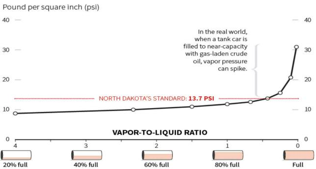
Note: Chart reflects vapor pressure readings of crude oil at different fill levels at 37.8°C/100°F. Sources: Ametek; Reuters.
